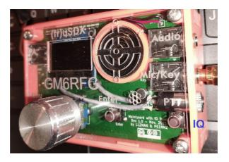
**Instructions:** Prepare two sections of miniature coax with no more than a 2mm diameter. For (tr)usdx these will pass through holes in the PCB to connect to a 3.5mm jack socket fitted to the case by the two existing PCB jacks. As shown in the photo below, prepare the coax and solder the braid to the ground and to the other coax section. Fit two 100nF ceramic capacitors two pins 7 & 1 of U9 as shown.
