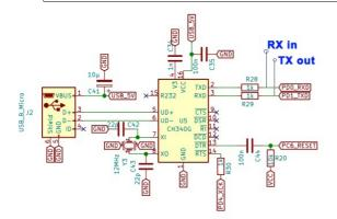
This modification supports both the USB and TTL RS232 com ports for direct connections to the Spectrum DSP module. This allows the USB com port on the Spectrum DSP to bypass CAT data to a connected PC or tablet.
